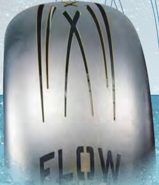
A water jet from Flow International was used to create this design on a motorcycle fender.
